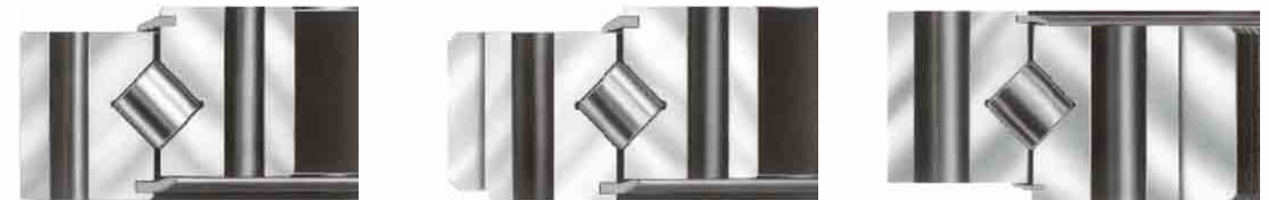
Single Row Crossed Roller Structure
